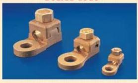
Bolted Copper alloy Lugs are a quick and easy way of making a connection on a normal or flexible conductor. Palms are machined top and bottom for bolting on either surface. They can be reused multiple times. Barrels have internal corrugations in the clamp to assist with current transfer.
