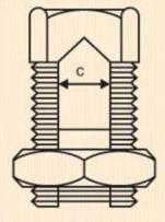
CONEX manufactures a vast range of Line Taps / Split Bolts / Cable Connectors to meet the material and dimensional specifications laid by different International Standards. Threads are formed by rolling process giving the nut extra clamping force. Pressure pads are made from extruded bars, preventing the pads from cracking. Line Taps are also offered with Copper palms and spacers (to separate dissimilar conductor materials and avoid corrosion).
