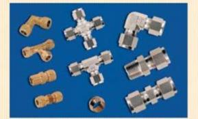
They are intended primarily for use in above and below ground water systems, central heating, hydraulics & pneumatics. They enable light gauge Copper, S.S., Polyethylene & PEX tubes to be well connected and consist of body with built-in stop for reclining of body with built in ring / ferrule corresponding size to the exterior diameter of tube and a compression nut. Single & twin ferrule fittings in Stainless Steel are also available.
